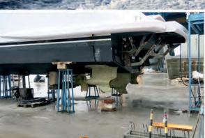
▲ Multiple IPS drives, in threes and fours, are becoming more common due to easier installation and improved performance
