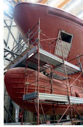
▲ Ice-busting steel is the material of choice for explorer yachts, such as this 500 EXP taking shape in Viareggio
