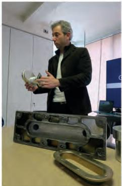
▲ Custom specialists Rossinavi design and manufacture many of their components for their unique builds, such as this bollard. Note the sculpting of the underside to reduce weight
