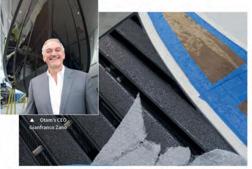
▲ Strong, lightweight carbon composites are finding many uses aboard. Here is Otam's carbon bathing platform on their Otam 80HT
