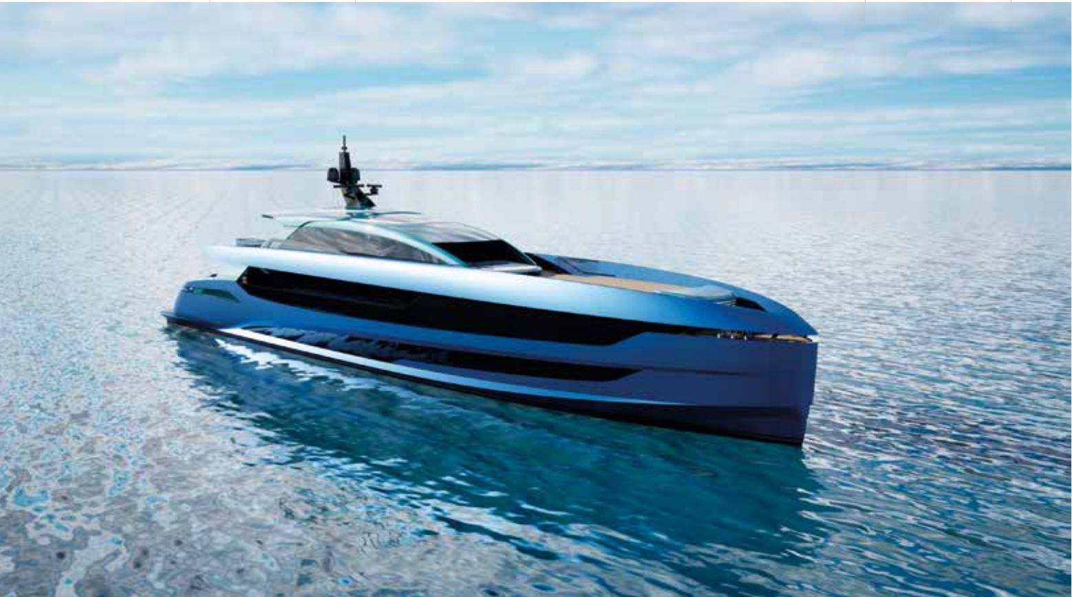
Above, the exterior of the AL50 RV, 50 metres long with a vertical bow. Below and opposite page, the AL50 RVF, the version with a fly bridge. Below, left, the design of the helm station with reverse windscreen and side windows that follow the coach house and shelter the sunpad area
